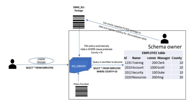
The above diagram shows how Fine Grained Acces Control(FGAC) works on an hypothetical table.
