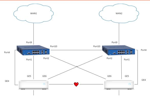
Port 4 to GE6: Management port connection Port 2 to GE6 - Circuit connection Port 10 to Port 10 - Trunk port connection GE6 to GE6 - SD-WAN (Velo cloud) connection
